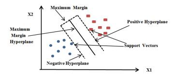
Fig-2:Support Vector Machine Classifier
