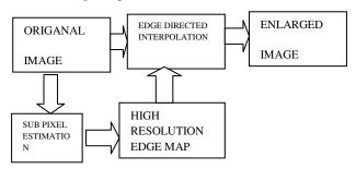
FIGURE 1 Edge directed interpolation structure
