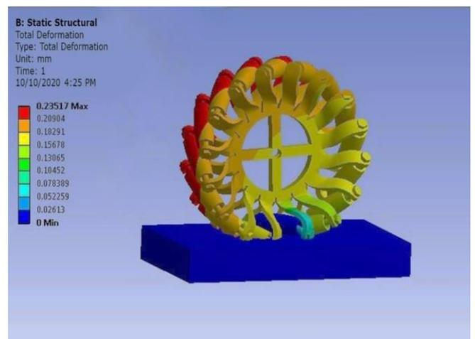
Fig 16: Deformation Undergone By Aluminium Alloy
