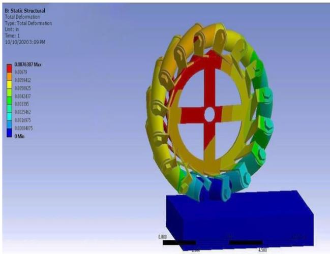
Fig 11: Deformation in Structural Steel
