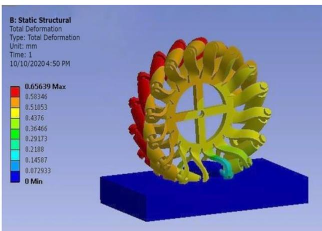
Fig 13: Deformation Undergone By Structural Steel
