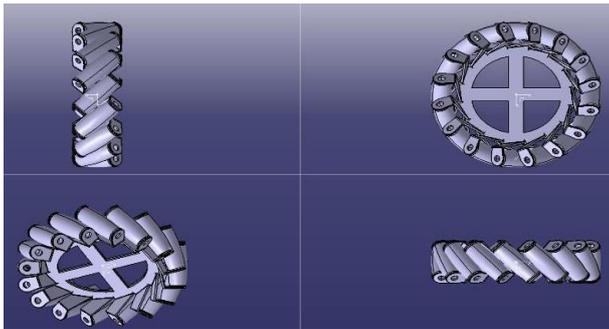
**Fig 6:** 4-View of Mecanum Wheel Designed In GSD WORKBENCH
