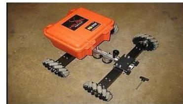
**Fig.1:** Mecanum Wheels Mounted on Robot Manufactured by Helical Robotics
