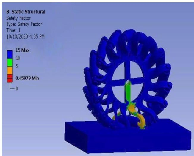
Fig 18: Safety Factor Noticed in Wheel for Aluminium Alloy
