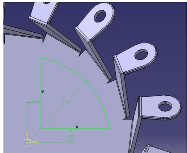
Fig 5: Design and Dimension of Pad and the Dimension of the Quadrant
