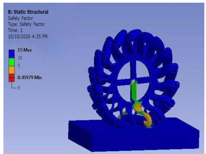
Fig 15: Safety Factor Noticed in Wheel for Structural Steel
