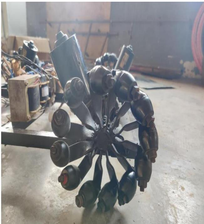
**Fig19:** Working Model of Mecanum Wheel
