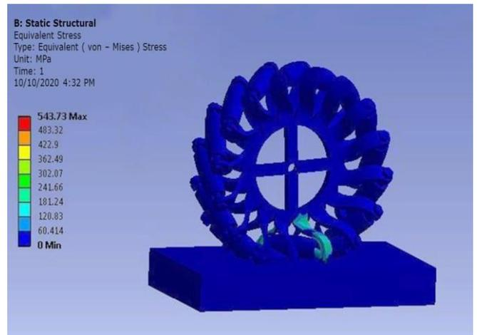
Fig 14: Equivalent Stress Distribution in Structural Steel
