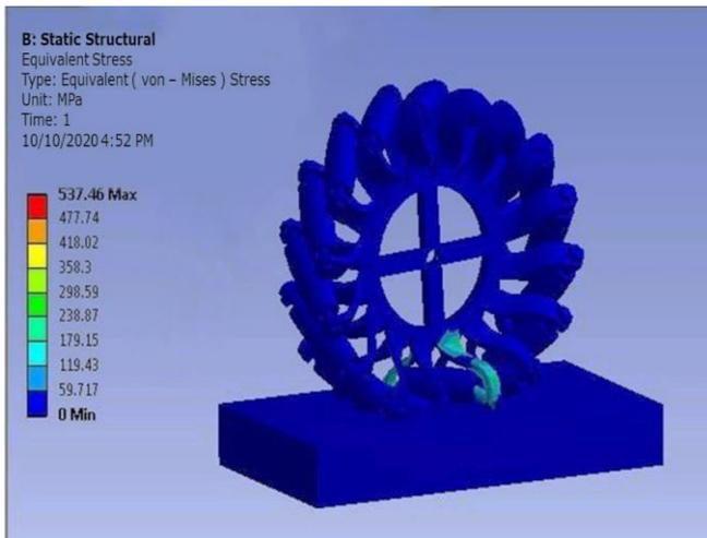
Fig 17: Equivalent Stress Distribution in Aluminium Alloy
