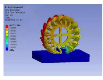
Fig 16: Deformation Undergone By Aluminium Alloy
