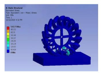
Fig 14: Equivalent Stress Distribution in Structural Steel
