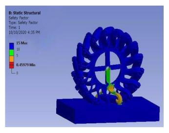
Fig 15: Safety Factor Noticed in Wheel for Structural Steel
