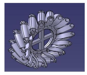
Fig 7: Modified Mecanum Wheel 1 Designed in CATIA
