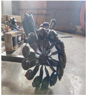
Fig19: Working Model of Mecanum Wheel
