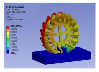
Fig 13: Deformation Undergone By Structural Steel
