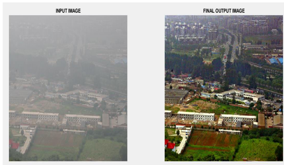
Figure 1 Input hazed and the output dehazed image obtained with our proposed method
