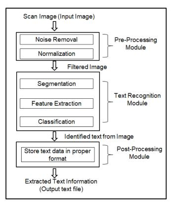
Fig. 6.1 Basic Architecture of text recognition system
