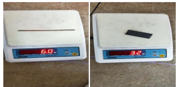
Fig. 3. Weight measurement of work piece and electrode
