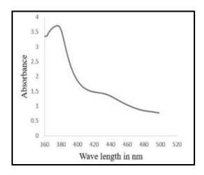
Fig 1 UV-Visible spectrum of zinc oxide nanoparticles
