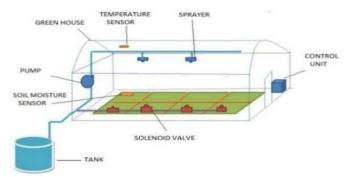
Figure 9: Structural Initialization
