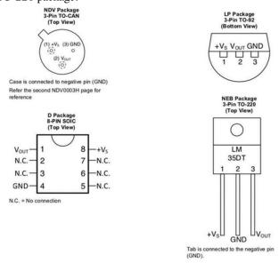
Figure 4: Temperature Sensor (LM35)
