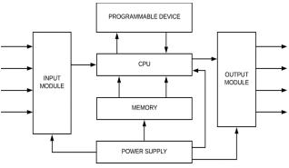
Figure 3: Block Diagram of PLC
