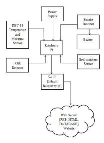
Figure 1. Block diagram of Green House Monitoring System
