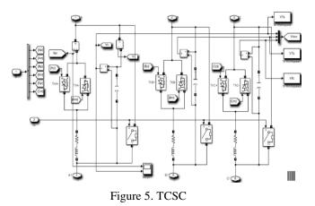
ThreeTCSCareconnected in three phases in transmis sion line in each phase. In addition, this TCSC firing angle are control and then the capacitor is variable in this TCSC, This TCSC are connect in center of the transmission line. Show in figure
