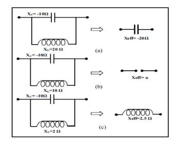
Figure 2. Basic characteristics of TCSC
