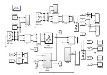
Figure 3. Simulink model of compensated system (With TCSC)
