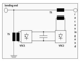
Figure 1: Basic diagram for UPFC
