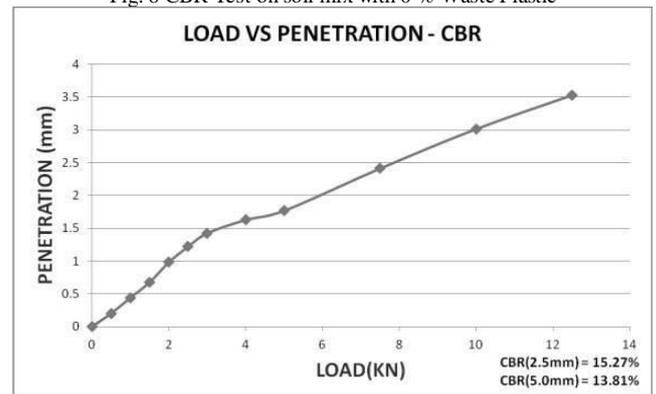
Fig. 9 CBR Test on soil mix with 0.25 % Waste Plastic
