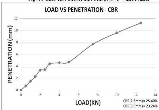
Fig. 12 CBR Test on soil mix with 1.0% Waste Plastic
