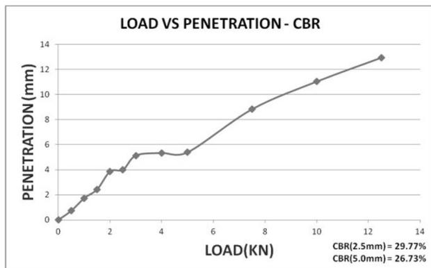
Fig. 11 CBR Test on soil mix with 0.75 % Waste Plastic
