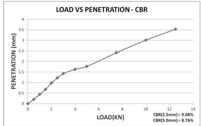
Fig. 8 CBR Test on soil mix with 0 % Waste Plastic
