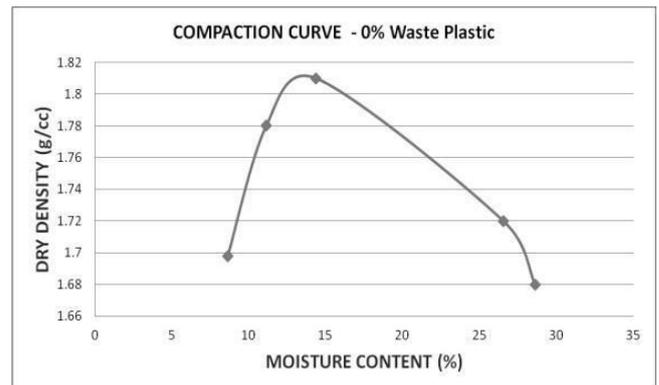
Fig. 3 Compaction curve for soil with 0% plastic
