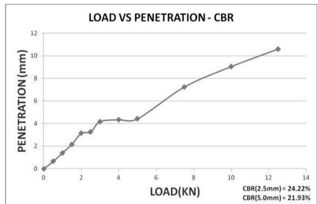
Fig. 10 CBR Test on soil mix with 0.5 % Waste Plastic
