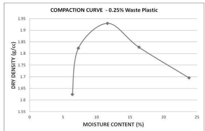
Fig. 4 Compaction curve for 0.25% Waste Plastic
