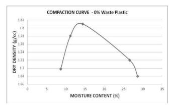
Fig. 3 Compaction curve for soil with 0% plastic
