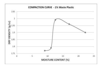
Fig. 7 Compaction curve for 1.0% Waste Plastic
