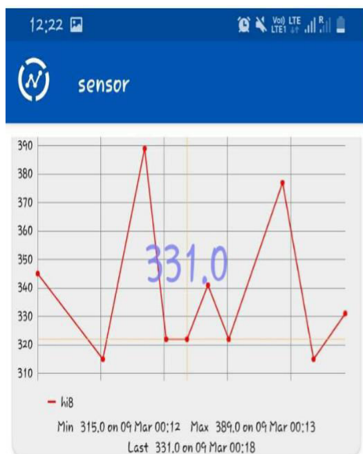
Figure 4.1 ESP8266 output for ultrasonic sensor.
