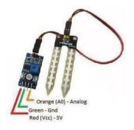
Fig 5: Soil Moisture Sensor
