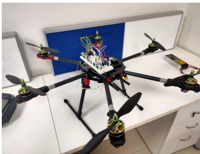
Fig 2: Hardware setup of Hexacopter.
