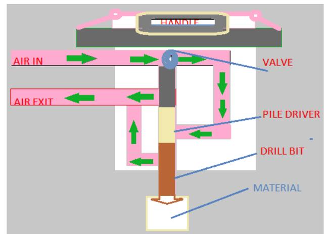
Fig 2 Schematic Diagram Pneumatic Drill Machine
