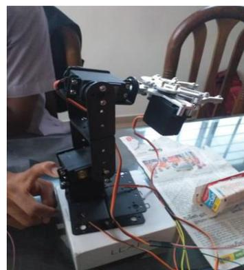
Fig -3: 4- DOF Robotic Arm
