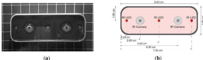
Fig -2: Leap Motion Controller
