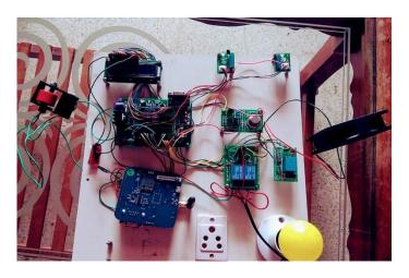
The model implemented for Industry monitoring using microcontroller and different sensors.
