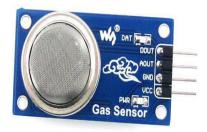
The Gas Detection system use the sensor of the MQ-2, the MQ-2 is used to detect the presence of Gas leakage (air pollution) and the signal gotten from the sensor are sent to the microcontroller and the status of the system is displayed on an LCD. With the help of the GSM module, the system sends SMS to the owner phone number telling the user the status of the environment whether a gas is detected in the industries surroundings.
