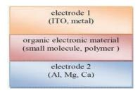
Fig 2: Basic structure of plastic solar cell
