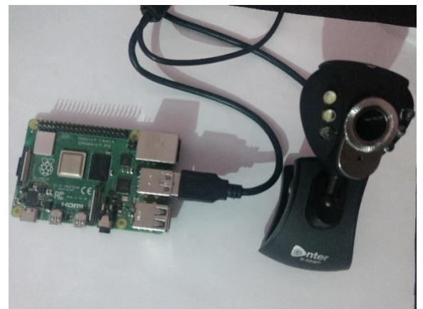
Fig 3.5 Connecting Camera Module to Raspberry Pi
