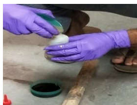
Fig-5: Mixing of polyol and isocyanate
