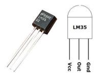
• The LM35 series of temperature sensors are produced by National Semiconductor Corporation and are rated to operate over a -55 °C to 150°C temperature range. These sensors do not require any external calibration and the output voltage is proportional to the temperature. The scale factor for temperature to voltage conversion is 10 mV per °C.
