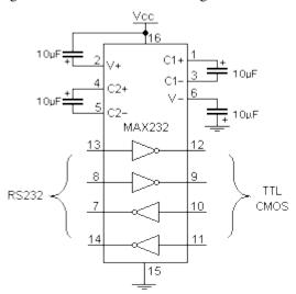
• The schematic shows the simplicity of the design by using one of IC's level converters. It includes a Charge Pump, which generates +10V and -10V from a single 5v supply. This IC also includes two receivers and two transmitters in the same package. This is handy in many cases when you only want to use the Transmit and Receive data Lines. You don't need to use two chips, one for the receive line and one for the,
