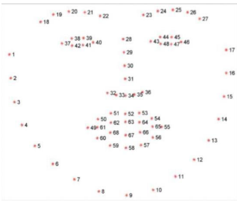
Fig 3- Facial Landmark Points according to Dlib Library
