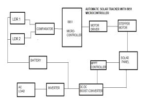
Fig. 1 Schematic representation of Solar Tracking System
