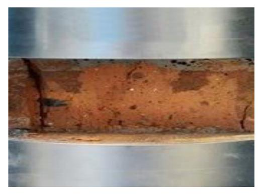
Fig.4.4 Testing Of brick Under CTM
