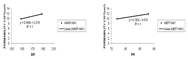
Figure 4.Effect of Fabric Weave Density on Formability with warp way and weft way (for plied yarn)
