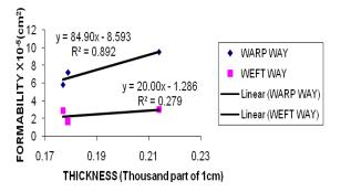
Figure2. Effect of fabric thickness on Formability with warp way and weft way
