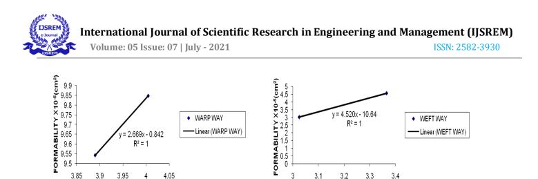
Figure3. Effect of Bending Length on Formability with warp way and weft way
