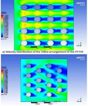
b) Velocity Distribution of the staggered arrangement of the PFTHE
