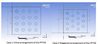
Fig -1: Arrangement of Tubes in PFTHEs
