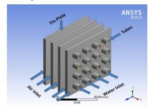
Fig -2: Model of the Inline PFTHE arrangement
