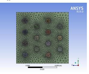
Fig -3: Meshing of the Staggered PFTHE model
