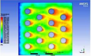
b) Temp. Profile of the staggered arrangement of the PFTHE
