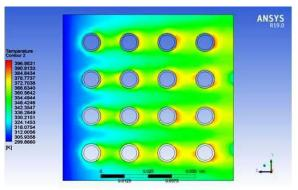
a) Temp. Profile of the Inline arrangement of the PFTHE
