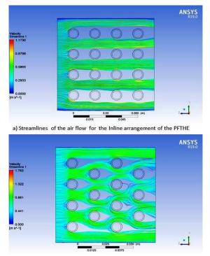
b) Streamlines of the air flow for the staggered arrangement of the PFTHE
