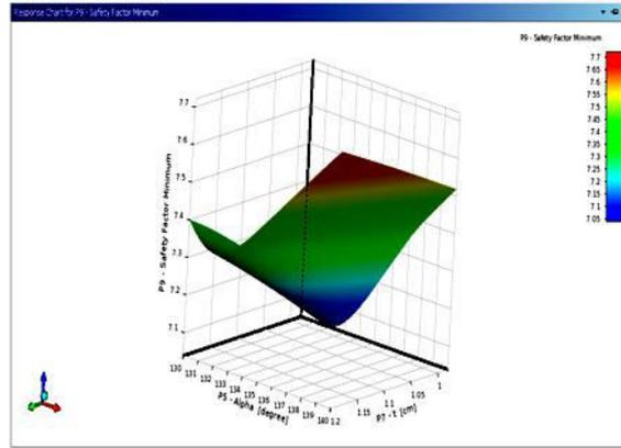
Figure 10: 3D response surface plot of Safety factor versus  $\alpha$  and h
