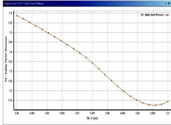
Figure 7: Safety factor versus h plot
