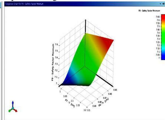
Figure 9: 3D response surface plot of Safety factor versus t and h
