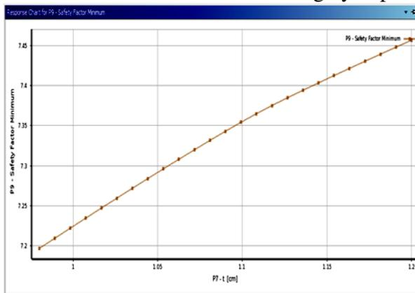
Figure 8: Safety factor versus t plot
