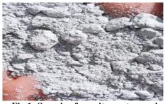
Fig 1: Sample of granite waste powder
