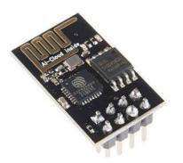
Fig.3 ESP8266 Board [10]
