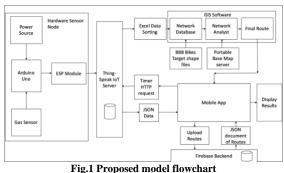
The proposed system will consist of a power source, an Arduino uno board, a wi-fi module ESP8266 and a gas sensor MQ-135 to measure the air quality. The wi-fi module will then send the data collected to the ThingSpeak IoT server for monitoring values in real time. Development of a mobile application will help the users see AQI values in real time.
