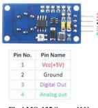
Fig.4 MQ-135 Sensor [11]
