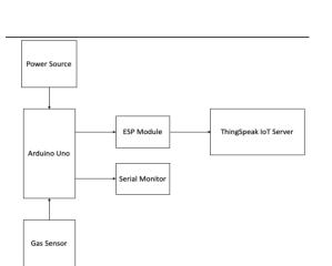
Fig.5 Hardware circuit flowchart
