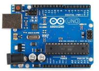
Fig.2 Arduino Uno Board [9]
