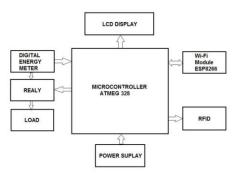
Fig. 1 Block diagram of proposed prototype smart energy meter
