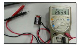
Fig. 5: Battery voltage measurement using multimeter
