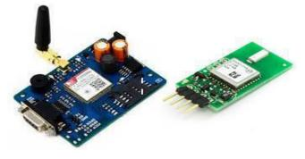
Fig.4: GSM and GPS Module
