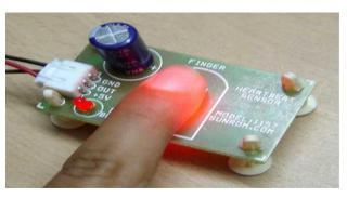
Fig.7: Heart Rate monitoring Sensor
