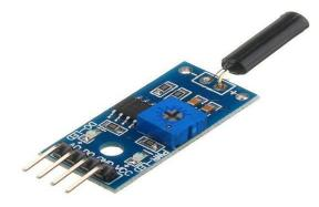
Fig.3: Vibration Sensor
