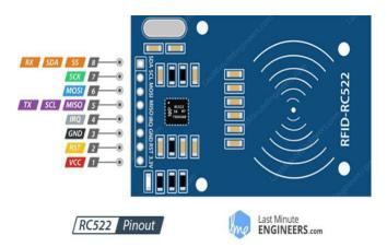
VCC supplies power for the module. This can be anywhere from 2.5 to 3.3 volts. You can connect it to 3.3V output from your Arduino. Remember connecting it to 5V pin will likely destroy your module!
