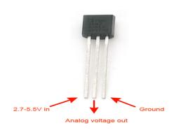
Fig -5: Temp Sensor(LM35)
