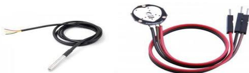
It is connect with Arduino and check continuously the body temperature and pulse rate of patient and display on LCD with which the doctors and other authorities can easily monitor the patient without human to human interaction.
