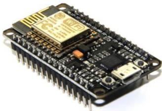
Arduino is in serial communication with the Wi-Fi module NodeMcu to connect with the internet and display real-time parameter from the cloud on blynk mobile app.
