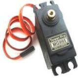
The Ambu-Bag compressing mechanism is operated with a servo motor which is connected to Arduino used for the compression and expansion of the ambu bag by its forward and reverse rotation.
