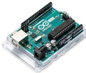
The arduino uno is a used as processor in our project. All the sensors, Wi-Fi module and servo motor will give input to the arduino uno and after getting input arduino uno will take process on it and gives output.
