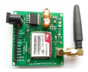
Fig 3.5 GSM MODEM
