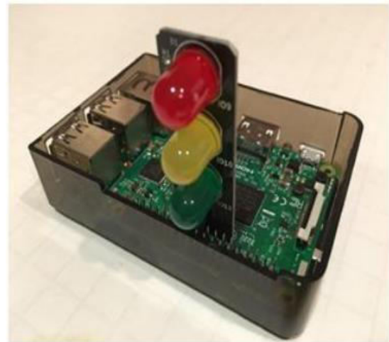
Fig: 3.3 Raspberry Pi integrated with three traffic LEDs
