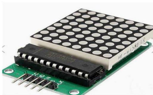
Fig -2: MAX7219 dot matrix display
