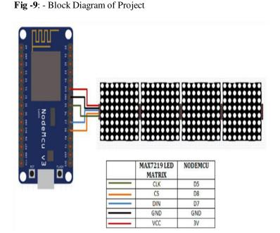
Fig -10: Schematic Diagram
