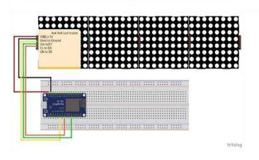
Fig -8: Connections between the LED matrix and ESP8266
