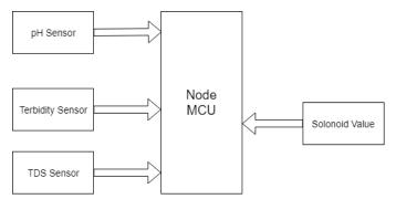
The Node MCU are accessing the sensor values and processing them to transfer the data through the internet. Arduino is used as a core controller. The sensor data can be viewed on the SMS system.
