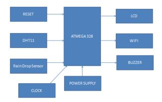
Using a Atmega 328 chip and a DHT sensor, you will develop an IoT based electronic device that streams temperature and humidity data over the internet. You can program the system in such a way that whenever there is a temperature/ humidity change, the system send the notification.
