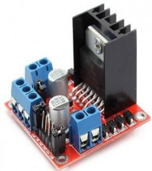
Fig.5.5 : DC motor driver
