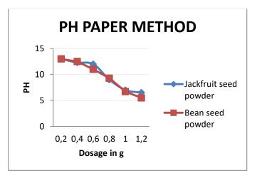
The pH of waste water quality standard as per BIS is 6.5-8.5. Initially when the wastewater is collected is found to be in Gejjalagere 15 after the treatment it will reduced to 7.5 for the dosage at 1 mg/l for Jackfruit seed powder and also it reduced to 6.7 for the dosage at 1g for Beans seeds.
