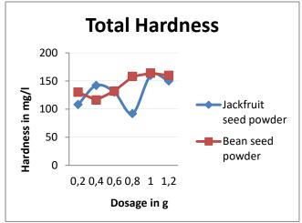
The Total Hardness of waste water quality standard as per BIS is 300 mg/l. Initially when the wastewater is collected is found to be in Gajjalagere 98 mg/l after the treatment it will reduced to 160 mg/l for the dosage at 1 mg/l for Jackfruit seed powder and also it reduced to 164 mg/l for the dosage at 1g for Beans seeds.
