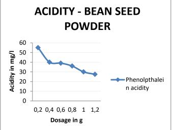
Acidity of waste water quality standard as per BIS is 0-100 mg/l. initially when waste water collected in Gejjalagere acidity is found to be 45mg/l after the treatment it will reduced to 0 mg/l for the dosage 1 mg/l for Jackfruit seed powder and also it reduced to 0 mg/l for the dosage at 1g for Beans seeds powder.
