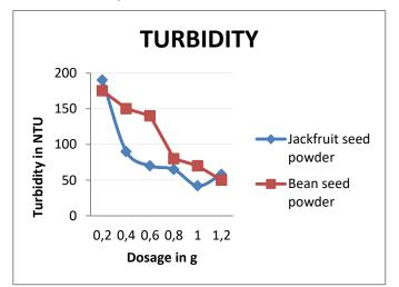
The Turbidity of waste water quality standard as per BIS is 10 NTU. Initially when the wastewater is collected is found to be in Gejjalagere 220 NTU after the treatment it will reduced 43 NTU for the dosage at 1 mg/l for Jackfruit seed powder and also it reduced to 70 NTU for the dosage at 1g for Beans seeds.
