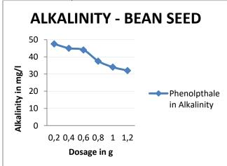
The Alkalinity of waste water quality standard as per BIS is 200-600 mg/l. Initially when the wastewater is collected is found to be in Gejjalagere 602 mg/l after the treatment it will reduced to 336 mg/l for the dosage at 1 mg/l for Jackfruit seed powder and also it reduced to 224 mg/l for the dosage at 1g for Beans seeds.
