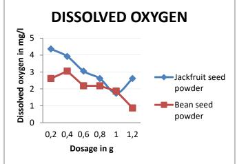
The Dissolved oxygen of waste water quality standard as per BIS is 5 mg/l. Initially when the wastewater is collected is found to be in Gejjalagere 6.45 mg/l after the treatment it will reduced to 1.74 mg/l for the dosage at 1 mg/l for Jackfruit seed powder and also it reduced to 1.87 mg/l (Gejjalagere) for the dosage at 1g for Beans Seed Powder.
