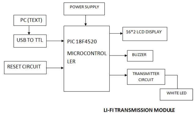
Fig -1: Block Diagram (Transmitter Section)
