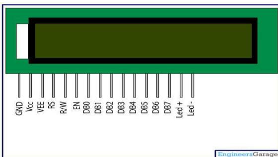
Fig -6: LCD Display
