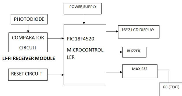
Fig -2: Block Diagram (Receiver Section)
