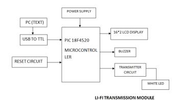
Fig -1: Block Diagram (Transmitter Section)
