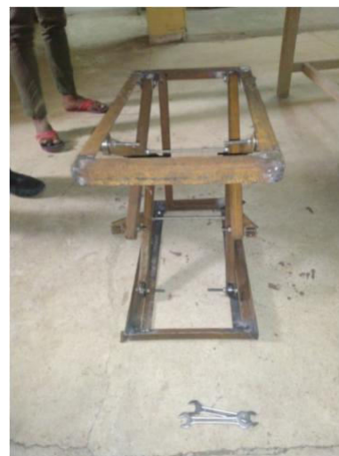
Figure-5: Sliding roller scissor mechanisms
