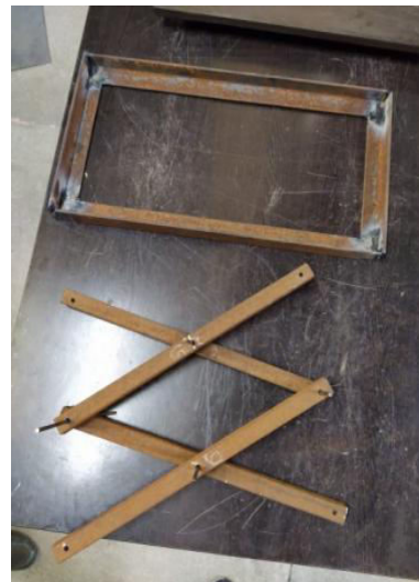
Figure-4: Frame and scissor pipe
