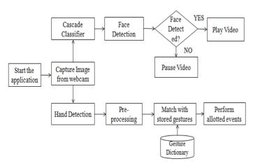
Figure: Architecture of the proposed system
